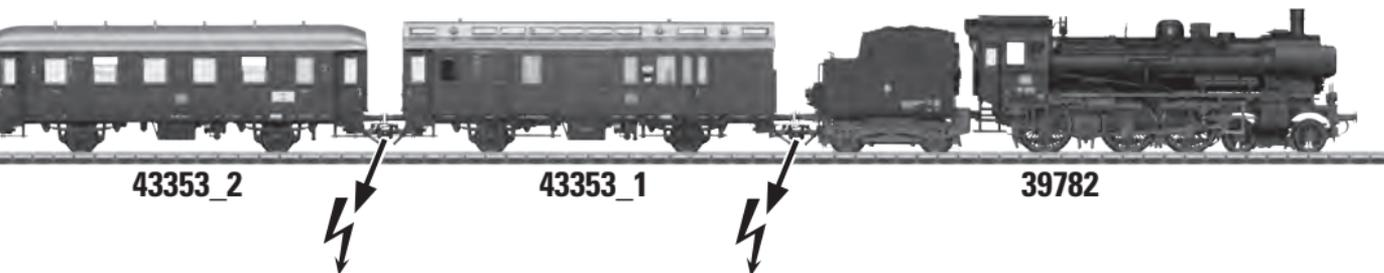
⚡ = stromführende Kupplung; current-conducting couplers; Accouplements conducteurs; Spanninggeleidende koppelingen; Conductoresde corriente; Conduitori di corrente; Strömledande kopplen; Stromforende koblinger
