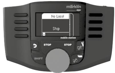
Place your locomotive on the track. After that, press the Stop button in order to turn power on to the track layout. After a short while mfx will appear on the display and will blink. This indicates that the locomotive is recognized and that the data is being read in.
