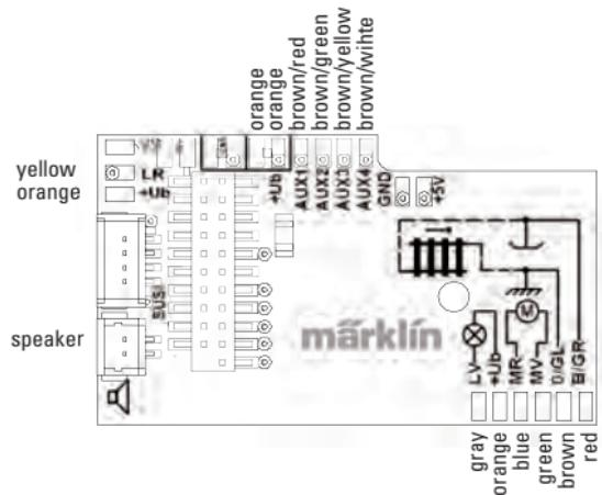
Insert the plug into the connector while paying attention to the positioning. Place the model, without body, on the programming track and test it. If the decoder works with no problems, the body can be put on the locomotive.
