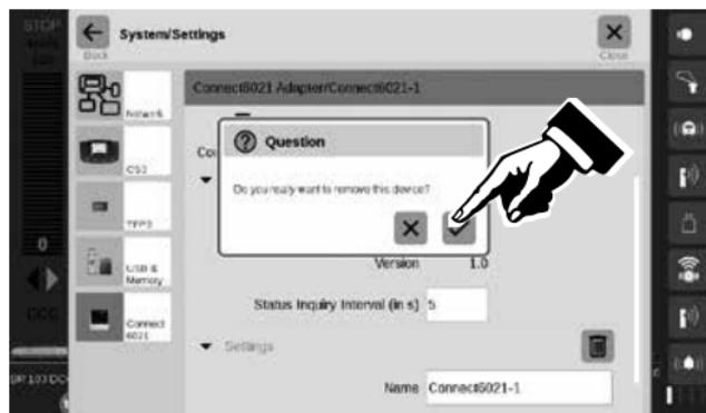
The Connect 6021 cannot be activated again until the Central Station has been started up again.
