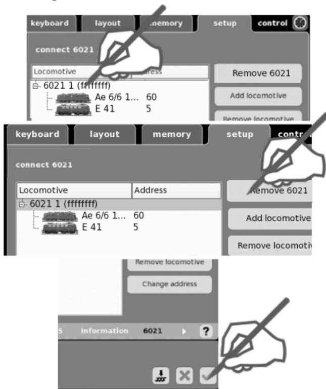
The Connect 6021 cannot be activated again until the Central Station has been started up again.
