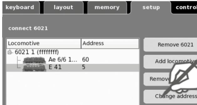
**!** Changing the converter address is not transmitted to the locomotive decoder!
