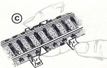
Mount current-feed clip from below as shown. Contact strip must make firm contact with base of rail.
